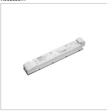
S.2422 POWER SUPPLY DIMMABLE DALI, PUSH DIM, DSI 100W 230Vac/24Vdc >1KHz IP20
