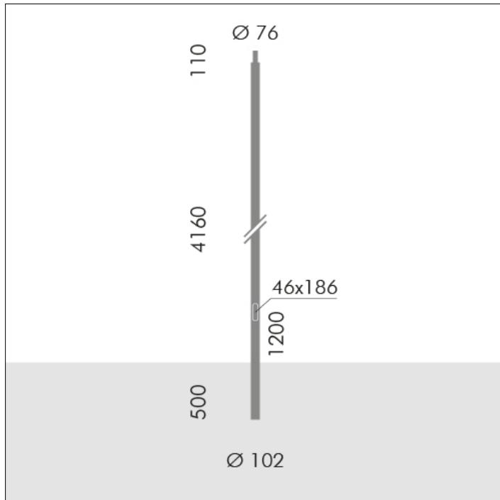
**S.2811****H 4,16m Ø102mm CYLINDRICAL POLE TO BE BURIED
