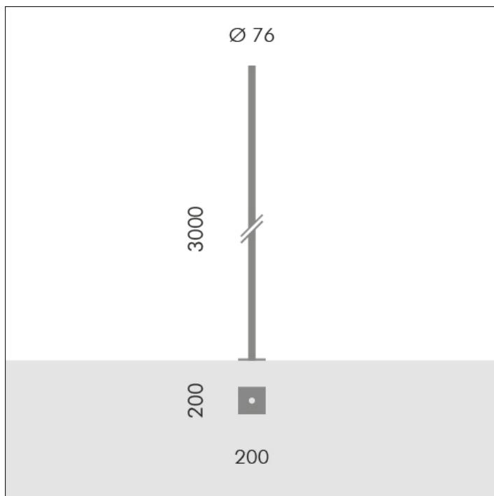
**S.2813****H 3,0m Ø76mm CYLINDRICAL POLE WITH BASE**
