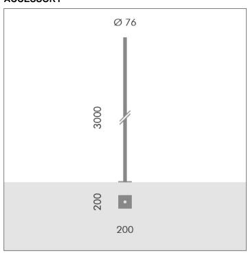
S.2813 H 3,0m Ø76mm CYLINDRICAL POLE WITH BASE
