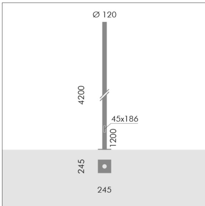
**S.2846****H 4,2m Ø120mm CYLINDRICAL POLE WITH BASE**
