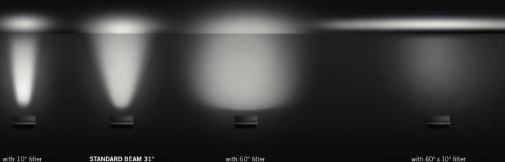
STANDARD BEAM 31° with 60° filter with 60° x 10° filter
