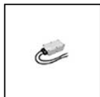
S.2493 IP67 Interface Virtual Midnight/Bilevel (Step-Dimming) This device is designed to maximize energy savings in various lighting applications. The devices can operate in two modes and are compatible exclusively with Simes DALI lighting fixtures: 1. Virtual Midnight: This system is designed for public outdoor lighting, enabling the automatic reduction of light output during periods when full-power operation is unnecessary. Configuring the system is straightforward, as programming is done via rotary selectors built into the device. 2. Bilevel (Step-Dimming): The two-level dimming system is commonly used in urban and street lighting, as well as in industrial facilities, emergency stairwells, parking lots, and other similar applications. The Bilevel function allows for adjusting the light intensity between two levels, using controls such as a relay, a twilight switch paired with a timer, or a motion sensor. The lighting level can be increased or decreased through simple programming using the rotary selectors built into the device. Dimensions 175.5mm x86.5mm x43mm It can manage a maximum of 7 DALI luminaires/devices. Possibility to extend up to max. 64 luminaires through the DALI Expander (S.2494).
